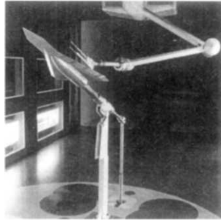
Fig. 1 LEX/Delta wing model in the test section of the KAFA subsonic wind tunnel
